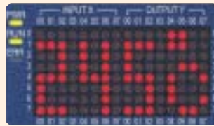
Display Mode 1: displays values, texts and graphics. User can designate 128 LEDs of the display as ON or OFF, so as to show various graphics in the display. Graphic or text cycling LEDs are also available.
