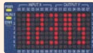
Display Mode 7: displays a five-digit value (0~32767). It displays the register's content value in the display. This mode is always used as the counter for finished goods or to demonstrate working hours.
