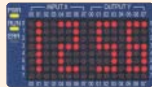
Display Mode 4: displays a two-digit value (00~99). It displays two register content values in the display for simultaneous observation on the change of these data.
