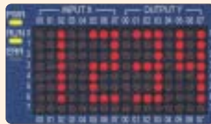
Display Mode 3: displays a four-digit value (0000~9999). It displays the register's content value in the display. This mode is always used as the counter for finished goods or to demonstrate working hours.
